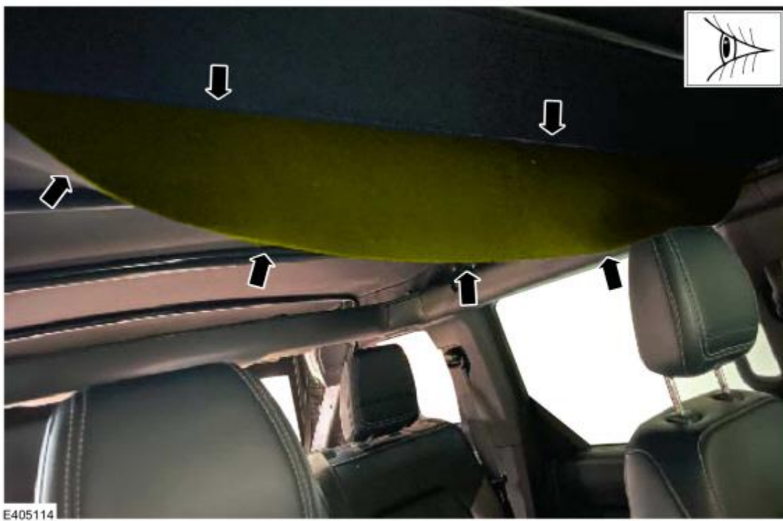
Figure 3 - Example of an undamaged, partially detached headliner that can be repaired
