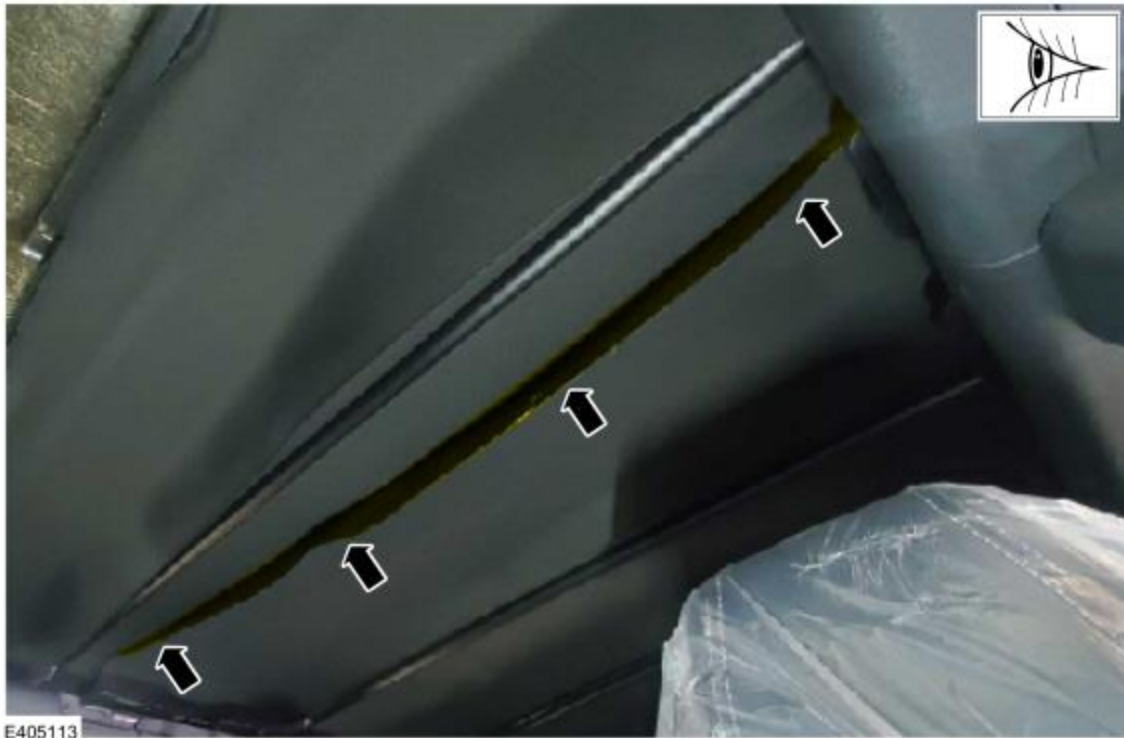
Figure 3 - Example of an undamaged, partially detached headliner that can be repaired
