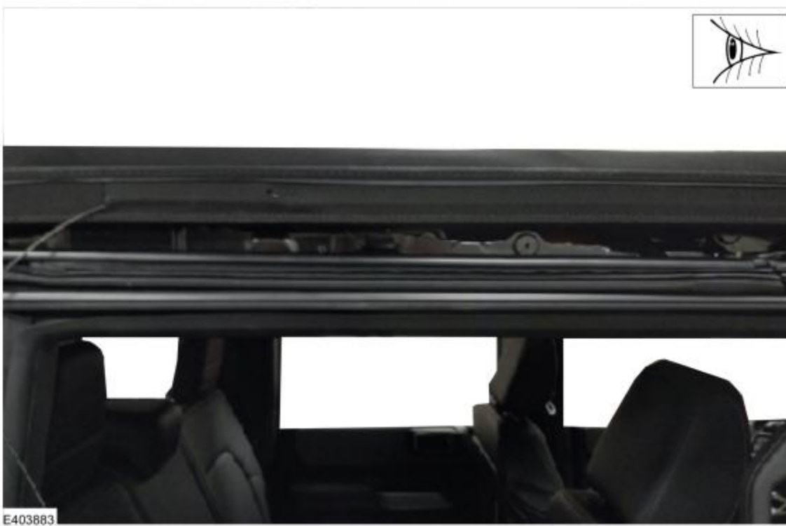
Figure 20 - Right side shown, left side similar. View of successful K-seal removal.
